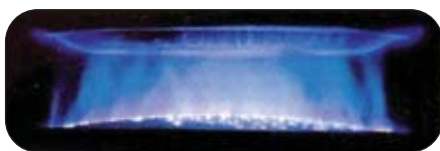
Axial Magnetic Field Interrupter - Arc Dispersion
